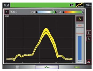
The Mandonic auto enveloping system adjusts the envelope limits perfectly according to the current variation of the process. The result: reliable detection of process errors with virtually no unnecessary machine stops. SKPuzzlemaster is provided for quick activation of additional expert monitoring routines.
